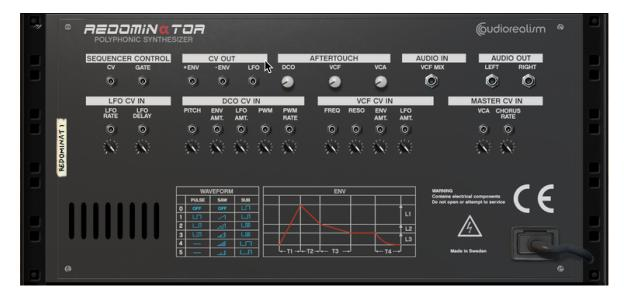
The back panel has several CV inputs and outputs which can be used to extend the control of ReDominator. There are also performance settings for aftertouch.
